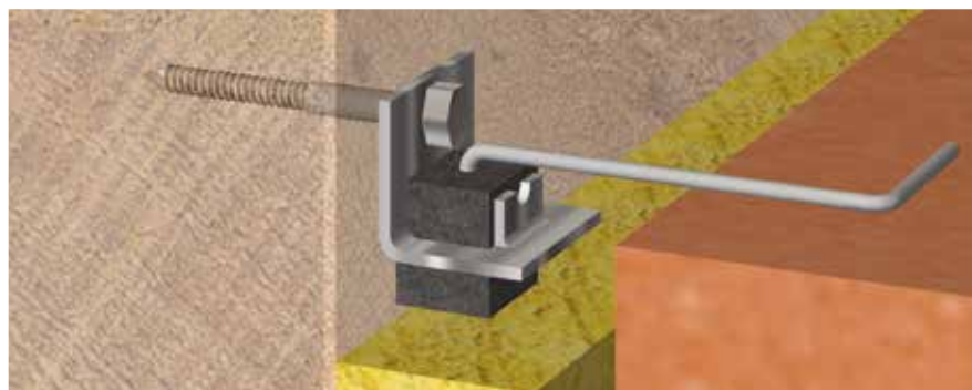
The end of the cavity tie must be visible along the underside of the acoustic block
